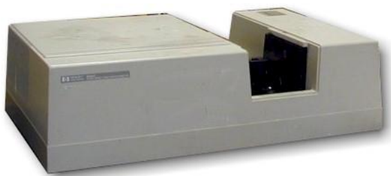
Fig. 2.1: Diagram of Hewlett Packard 8452A diode array spectrophotometer.
