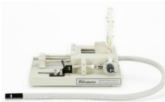
Fig. 2.2: Diagram of Photo-physics RX-2000 stopped flow accessory.
